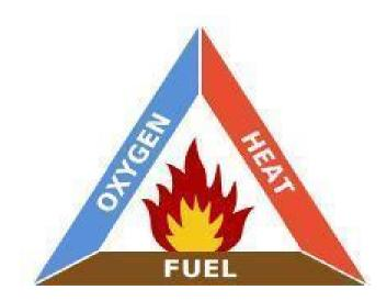
The triangle illustrates that a fire needs these three elements to ignite or burn, and will be prevented or extinguished if one is removed.
